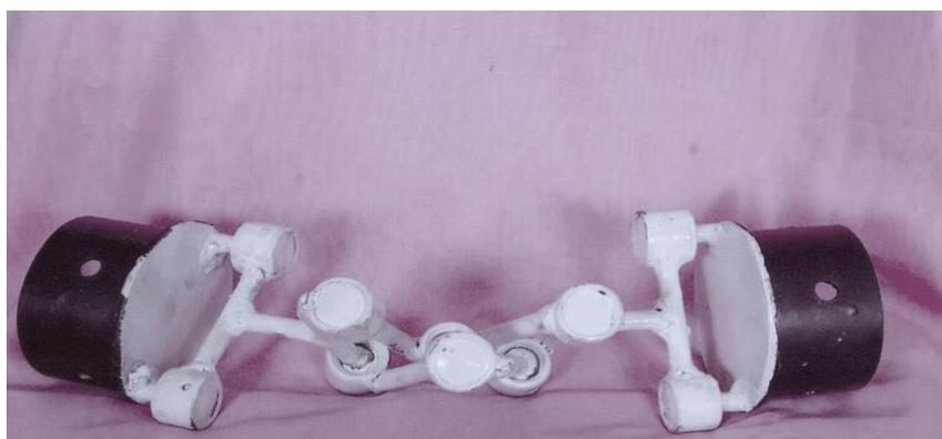
**Figure. 4.13. General view of the prototype lever-articulated coupling**
