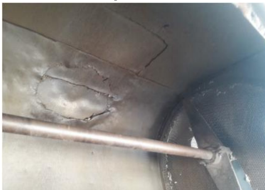
Fig.1.4. Internal view of the wall of the CC-15A separator after repair.
