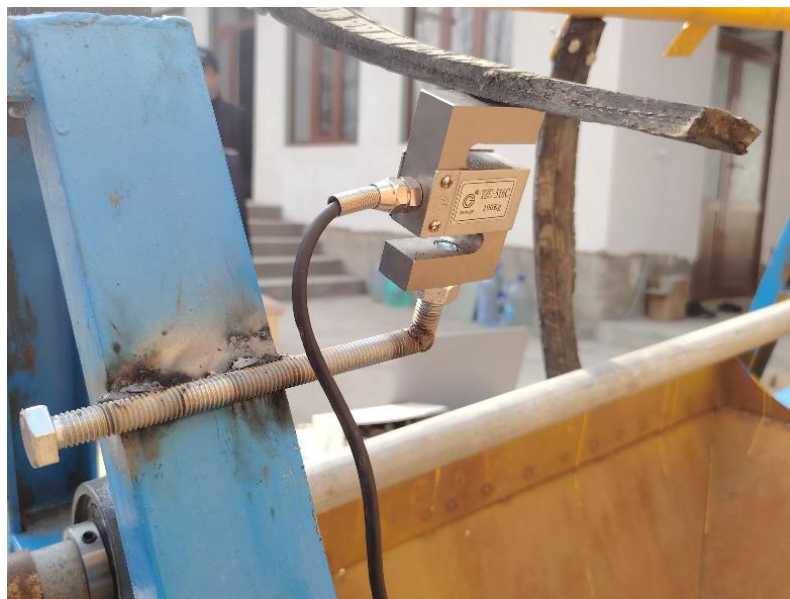
Fig. 3.3. YZC-516C strain gauge sensor (a), its calibration process (b)
