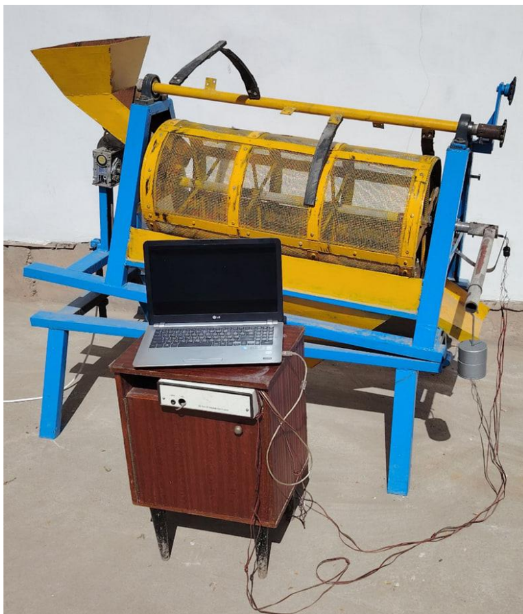
Fig. 3.8. Calibration process of the torque on the mesh drum shaft
